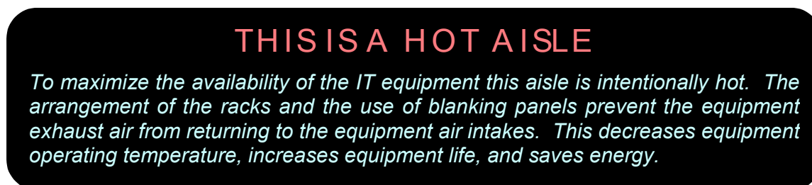
Figure 4 – Label communicating the purpose of the hot aisle
